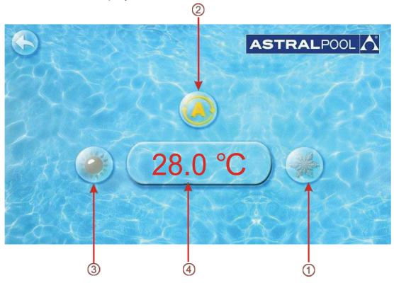
Click the refrigeration mode button ①, automatic mode ② or heating mode button ③then you can select the corresponding mode.
