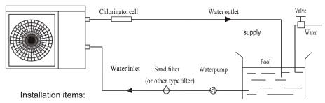
The factory only provides the main unit and the water unit; the other items in the illustration are necessary spare parts for the water system, that are provided by users or the installer.
