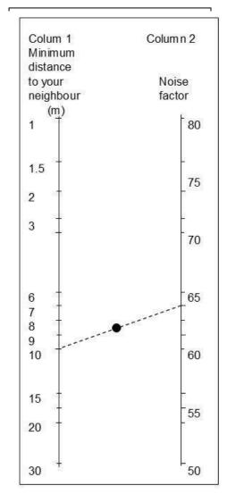
With one reflective surface and a timber paling fence with small gaps, the Heat Pump needs to be installed at least 10 metres from a noise sensitive area in your neighbour's property.
