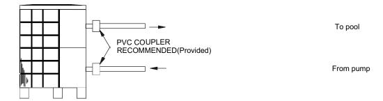
Condensation: Since the Heat pump cools down the air about 4 , water may condense on the fins of the horseshoe shaped evaporator. If the relative humidity is very high, this could be as much as several liters an hour. The water will run down the fins into the base pan and drain out through the barbed plastic condensation drain fitting on the side of the base pan.
