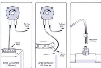
When inserting chlorine and acid tubes into dosing cell, tubes should penetrate approximately 50mm or half way into the depth of the mixing chamber. If the tube has a radius formed which is caused by the memory of the material, it is important that the tube point in the direction of the water flow.
