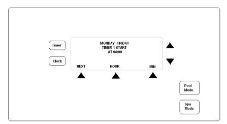
5. Using the up and down arrows in conjunction with the HOUR and MIN buttons, set the time you want the filtration pump to start at. Press NEXT when done.
