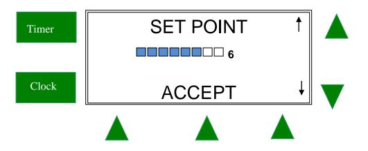
Use the up and down buttons to change the Set Point between 0 and 8. o chlorine output should only be used when there is no salt in the water. In summer, the chlorine should be set between 6 and 8 and you should regularly check your chlorine level in your swimming pool to determine if the output should be increased or decreased. Rely on your pool professional for advice on the recommended chlorine level in your pool.
