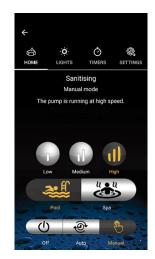
From this page you can turn the Chlorinator On, Off or to Auto, select Pool or Spa Mode and set the pump speed (if a compatible AstralPool pump is installed)
