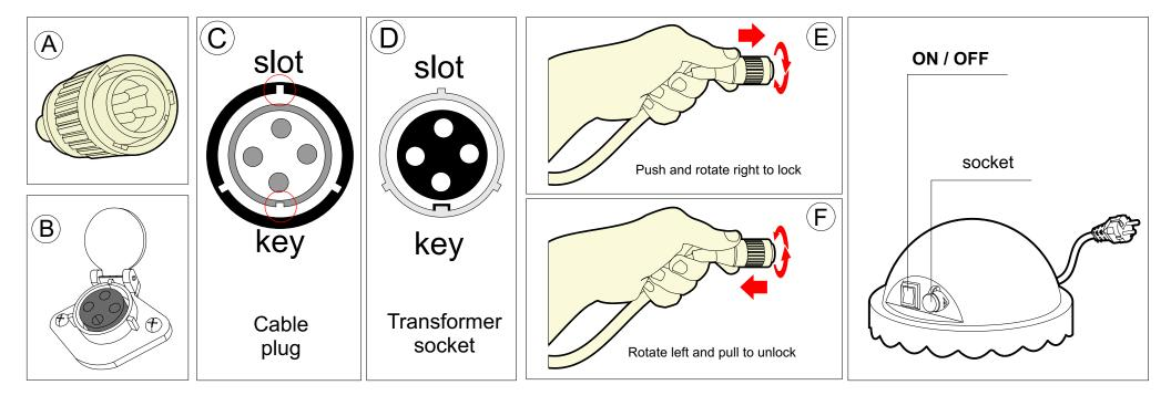
**To plug the cable** (Fig A) into the socket on the power supply (Fig B), please do the following:
