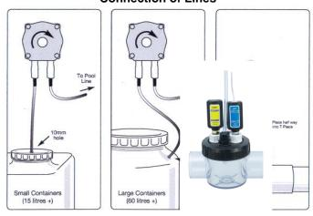
When inserting chlorine and acid tubes into dosing cell, tubes should penetrate approximately 50mm or half way into the depth of the cell. If the tube has a radius formed which is caused by the memory of the material, it is important the to tube point in the direction of the waterflow.
