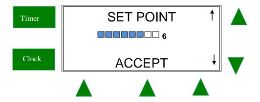
Use the up and down buttons to change the Set Point between 0 and 8. 0 chlorine output should only be used when there is no salt in the water. In summer, the chlorine should be set between 6 and 8 and you should regularly check your chlorine level in your swimming pool to determine if the output should be increased or decreased. Rely on your pool professional for advice on the recommended chlorine level in your pool.
