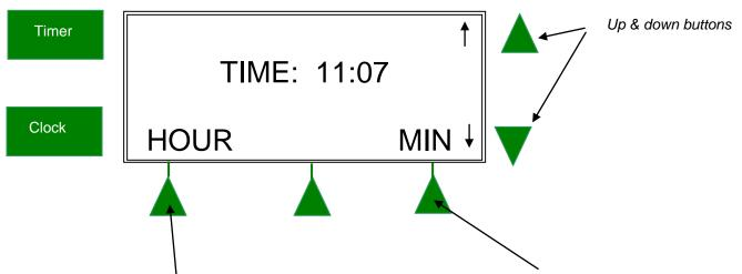
Select hour and use up or down buttons to change hour. Select Min and use up or down buttons to change the minute
